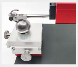
Measurement with measuring stand and a UH tracer with skid suitable for radial measurements on balls and pipes from  $\emptyset$  8 mm.
