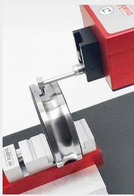
Measurement with measuring stand and a KKH tracer with skid suitable for concave and convex surfaces, e.g. ball bearing guide.
