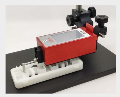
Measurement with measuring stand and a NH tracer with skid suitable for slots and deeper surfaces up to a maximum of 20 mm.
