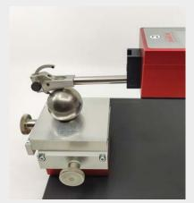
Measurement with measuring stand and a tracer KKH with skid suitable for concave and convex surfaces, for example ball bearing guide.
